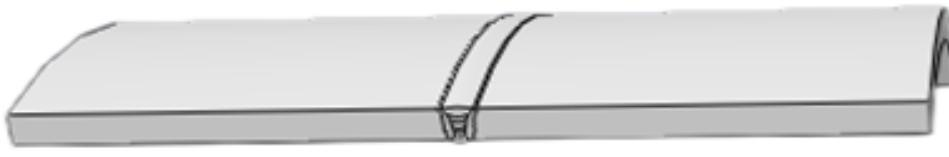
**Figure 4:** which illustrates the geometric model of the GMAW joint.
