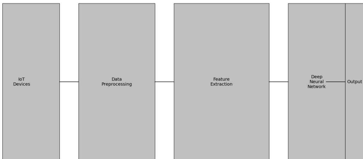
Figure 1: Architecture of the Proposed Deep Learning Framework for IoT Anomaly Detection
